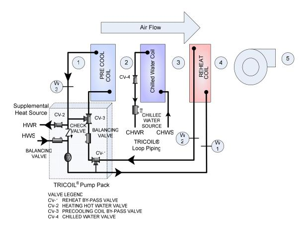
OPERATING SEQUENCE: The following notes are intended to provide a brief over-view of the operating sequence for the TRICOIL® VAV control.
